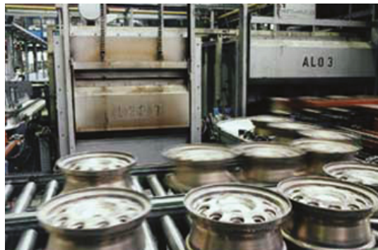
Aluminium industry: curing oven for wheel rims
